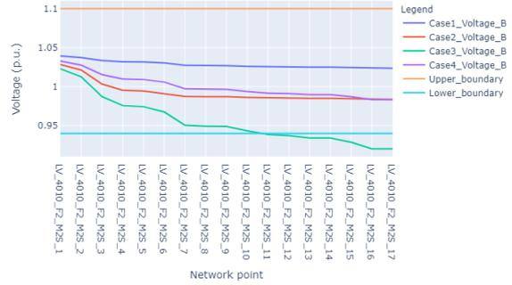
Figure 7: Voltage drop along a three phase LV main at the time of the highest power loss across all scenarios
