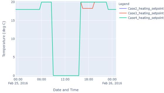
Figure 5: Heating set points for all scenarios (Note: Scenarios 2 and 4 are identical)
