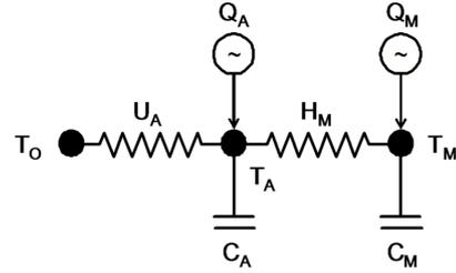
Figure 3: Equivalent Thermal Parameter Model implemented in GridLAB-D
