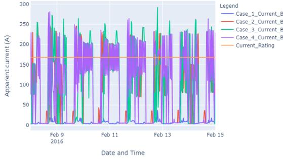
Figure 9: Underground cable loading for all scenarios
