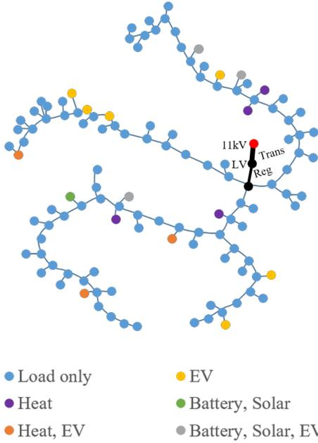
Figure 2: Network diagram of the LV section simulated.
