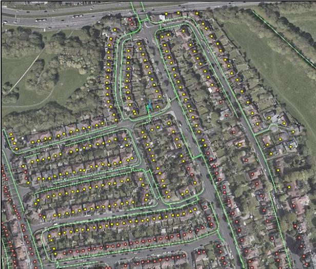
Figure 4: Areal and schematic view of domestic housing stock fed by one LV substation. As per real data provided by the Newcastle City Council.
