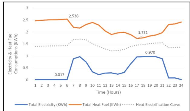
Figure 7: LV area January hourly average total electricity and heat fuel consumption in kWh
