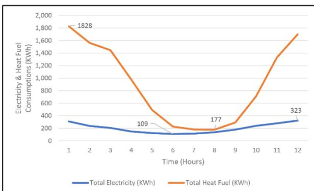
Figure 6: LV area monthly average total electricity and heat fuel consumption in kWh
