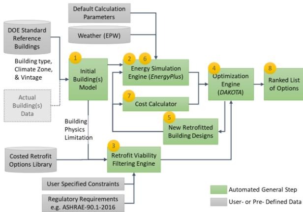
Figure 1: Automated process to maximize the building energy performance and minimize the investment cost
