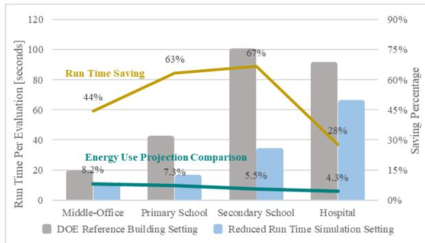
Figure 2: Comparison of savings in EnergyPlus run time and building energy use projection using proposed simulation parameter settings against DOE reference building parameters for four building use types
