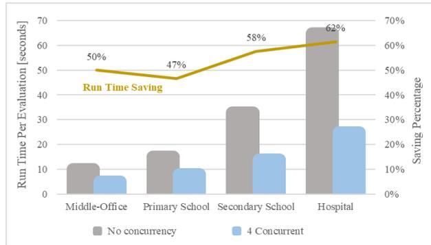
Figure 3: Comparison of savings in EnergyPlus run time when executing 4 concurrent simulations against no concurrency for four building use types
