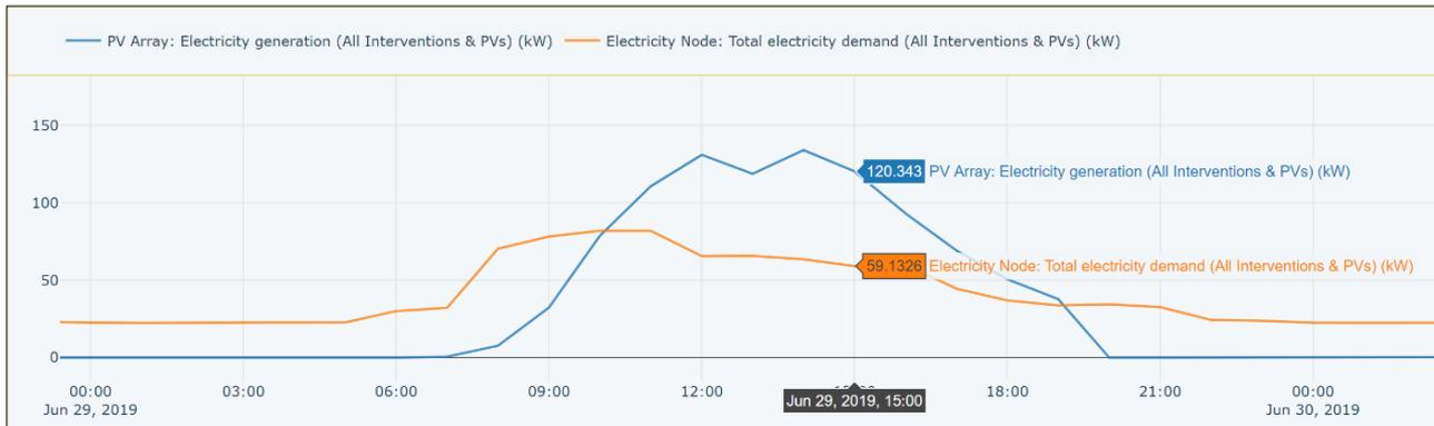
Figure 8: PEB energy demand and generation on a typical non-working day.
