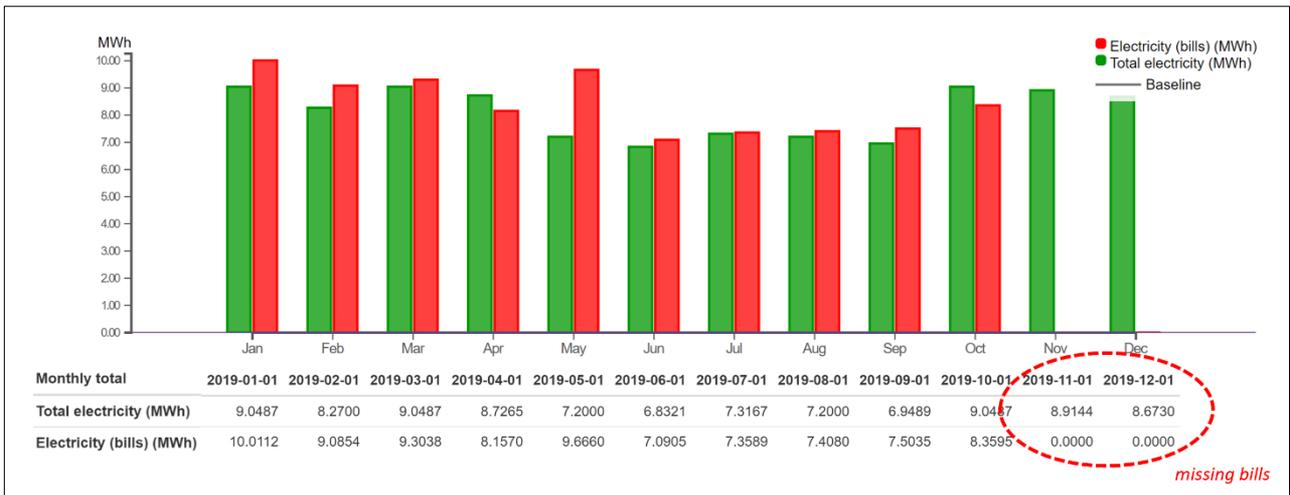
Figure 6: Comparison of real/simulated electricity consumption for Building 1.
