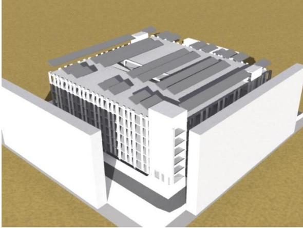
Figure 2: rendered model of the ESP-r Duke St Car Park model with roof-mounted PV arrays.
