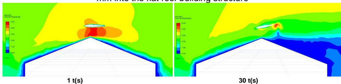
Figure 5. The velocity contour of an oscillating aerofoil integrated with a distance of 600 mm into the pitched roof building structure
