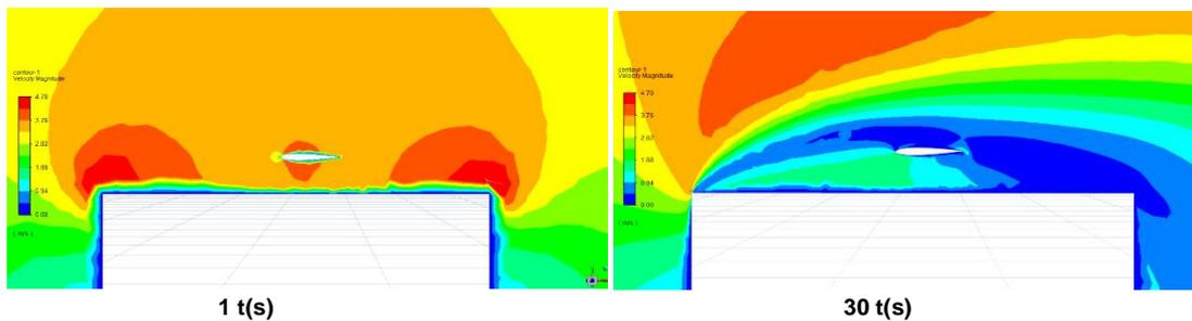
Figure 3. The velocity contour of an oscillating aerofoil integrated with a distance of 600 mm into the flat roof building structure
