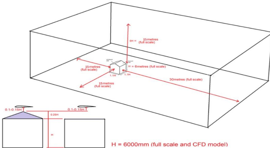
Figure 1. The dimension of the 3D computational model created in Design Modeler
