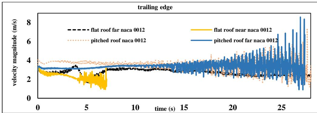
Figure 8. Velocity magnitude located at the trailing edge point of the aerofoil
