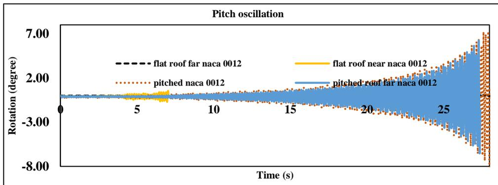
Figure 10. Pitch oscillations diagram for a speed of 3 m / s
