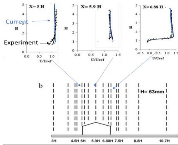
Figure 2. The comparison between numerical CFD results and experimental data (Ntinis et al., 2014)
