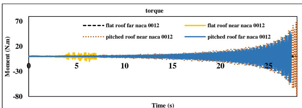
Figure 9. Torque diagram in pitch mode for a speed of 3 m / s
