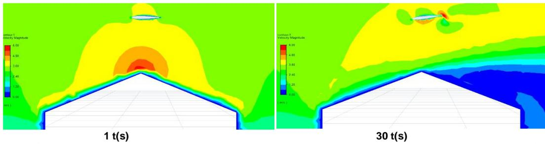
Figure 6. The velocity contour of an oscillating aerofoil integrated with a distance of 1200 mm into the flat roof building structure
