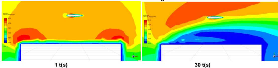
Figure 4. The velocity contour of an oscillating aerofoil integrated with a distance of 2,100 mm into the flat roof building structure
