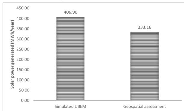
Figure 8 Annual solar power generated (MWh/year) comparison between the simulated model and geospatial assessment
