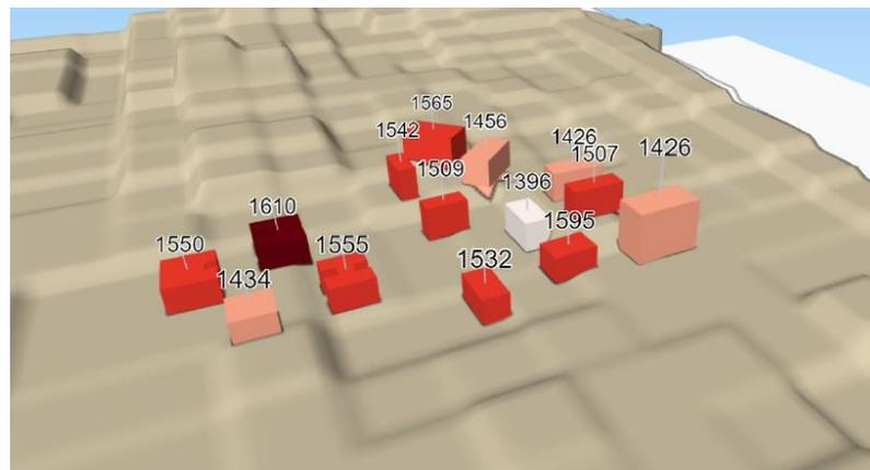
Figure 6 Visualization of the average annual horizontal radiation (kWh/m<sup>2</sup>/year) upon the rooftops in QGIS
