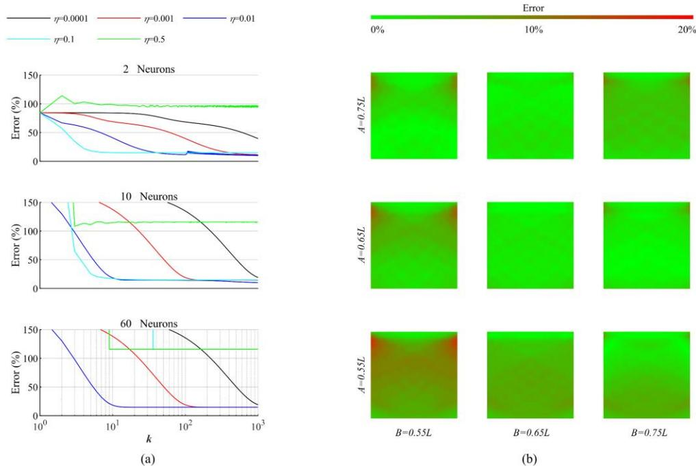
Figure 7. (a) Error variation with the number of iterations ( $k$ ) for different numbers of neurons in the hidden layer and different fixed step sizes ( $\eta$ ). (b) Error contours for the 9 testing points.
