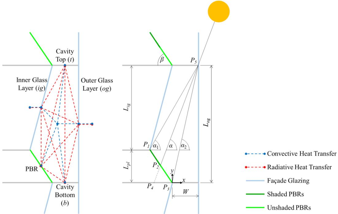
Figure 2. Left: Convective and radiative heat transfer modes of the DSF. Right: Parameters considered for investigating SF of PBRs integrated into DSFs.
