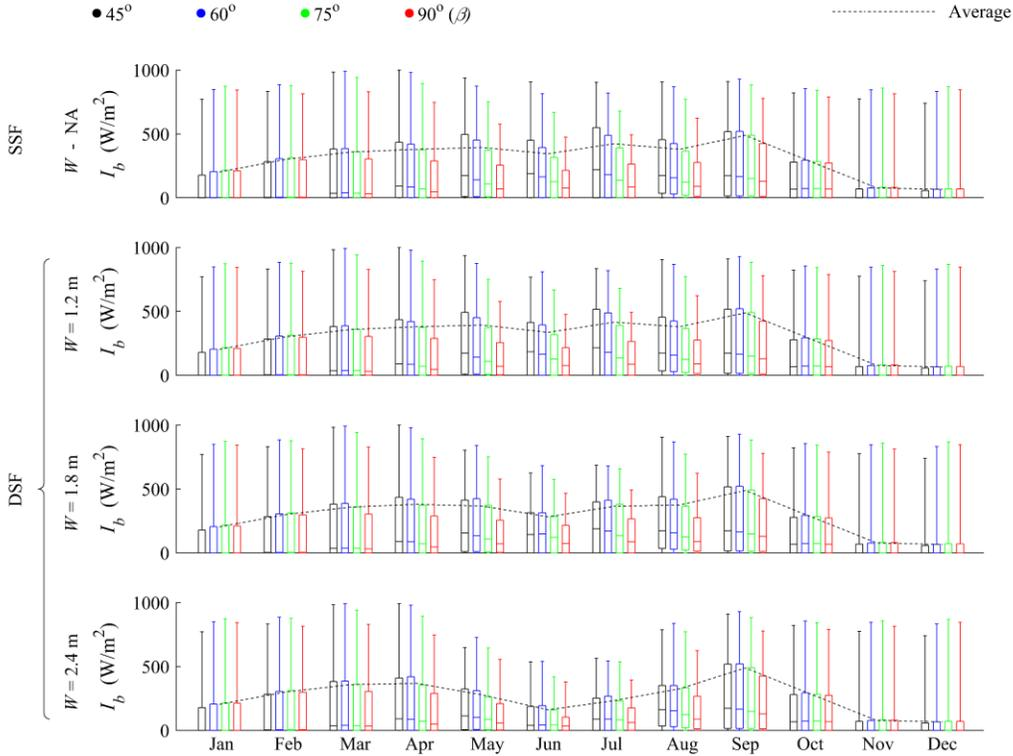
Figure 4. Variation of hourly  $I_b$  in each month for different façade systems and tilt angles.
