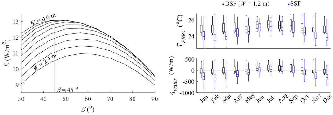
Figure 5. Left: Annual average  $E$  for DSF systems with different  $W$  and  $\beta$ . Right: Hourly variations of PBRs' wall temperature and generated/required heat for SSFs and the optimal DSF.
