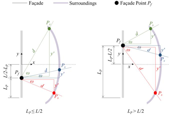
Figure 3. Plan view of the building façade and context for all possible combinations of  $\omega$  and  $L_p$ .
