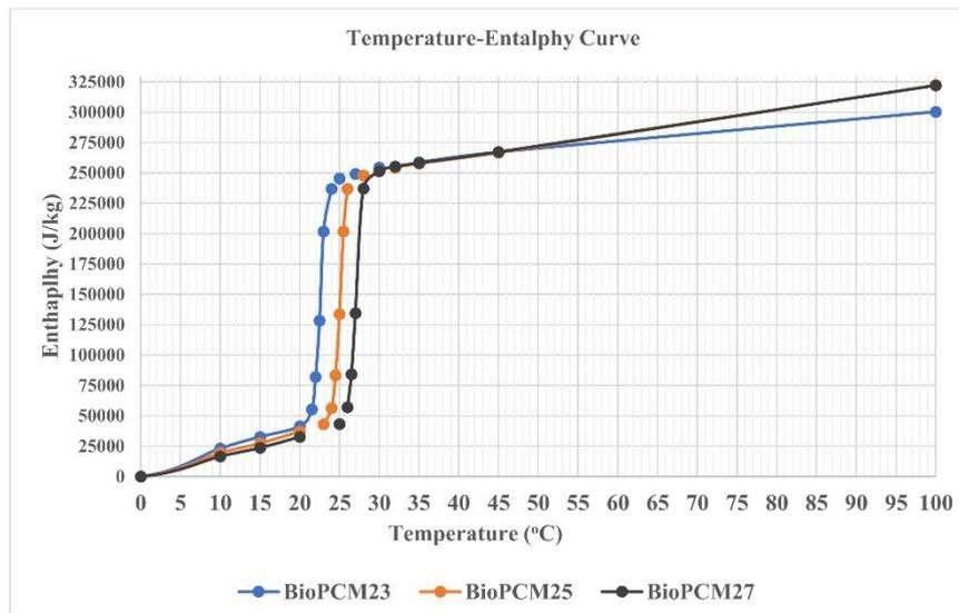
Figure 4. Temperature-enthalpy graphic of the PCM options (Designbuilder Database)
